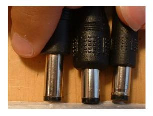
The problem was solved by switching the plugs around until all had a good connection and all wires to the power supply were plenty long. Oh, made sure the polarity was OK too. Bottom line. When powering equipment from a "junk box" 3.5mm plug, check its length.
